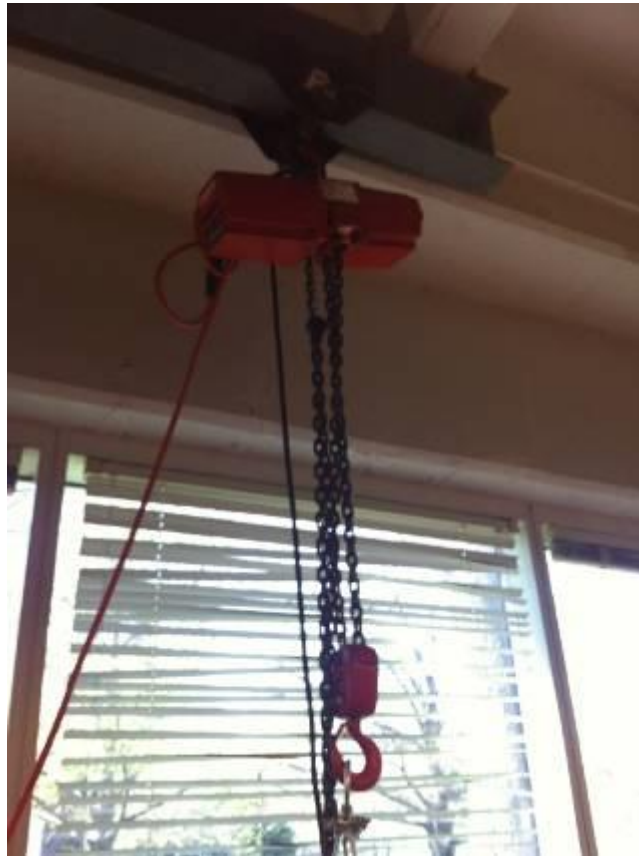
Figure B.8: 500 Lbs. crane
