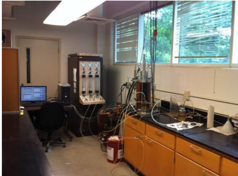
Figure B.1: Pressure board, hydraulic system, cyclic triaxial system and a personal computer
