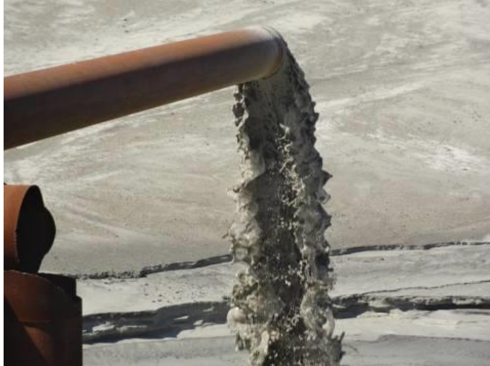
Figure 1.2: Wet disposal method
